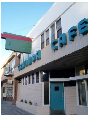
Left: Painted sheet metal individual letters of the Granada Cafe, built in 1949, on Mission Street in the Excelsior District. This largely intact storefront features additional Midcentury Modern design elements including a recessed, asymmetrical entryway, overhangs, brick veneer, and planters integrated in the building's façade. Right: The Butler Brothers department store (1952) at Stonestown featured a "billboard facade" with script lettering readable from an automobile. Photos: Mary Brown, San Francisco Planning Department; San Francisco History Center, San Francisco Public Library
