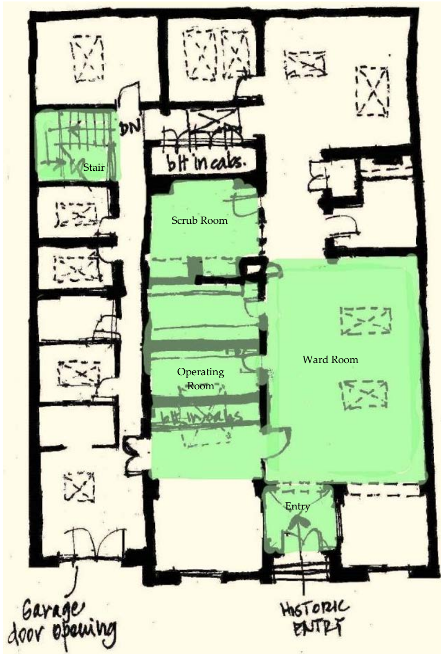
First floor plan; location of character defining features represented by green shading.
